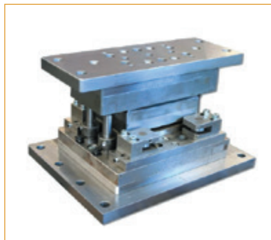
FIGURE 1. Hard punch and dies are complex and expensive tools that require precision machining, and near perfect alignment of the upper punch and lower die in order to produce good results on thin materials like flexible circuits. It is not uncommon for a flex circuit hard tool to weigh 100-200lbs.
