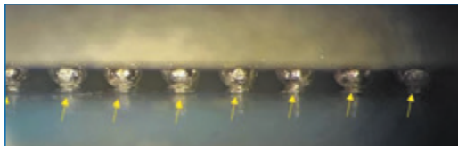
FIGURE 16. Side B solder balls before VPS rework.
