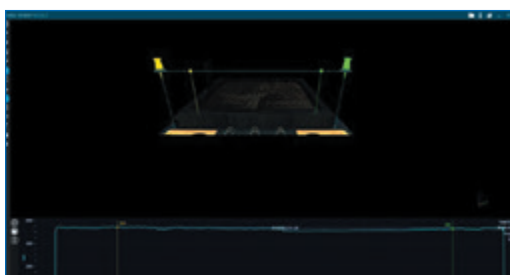
FIGURE 13. 3-D AOI rendered image of side D after rework. Calculations made by pins seen in image.
