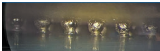
FIGURE 18. Side C solder balls before VPS rework.
