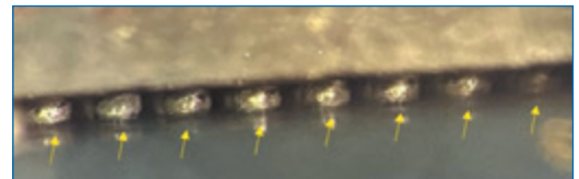
FIGURE 17. Side B solder balls after VPS rework.
