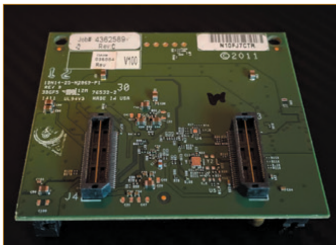
FIGURE 3. A similar board with the infamous stacking connector pair that brought the design to a standstill.
