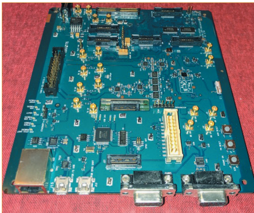
FIGURE 1. A mixed-signal board is always a stretch, with the various functions vying for limited space.
