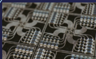
This image shows circuitry formed with SW series on glass substrate.
