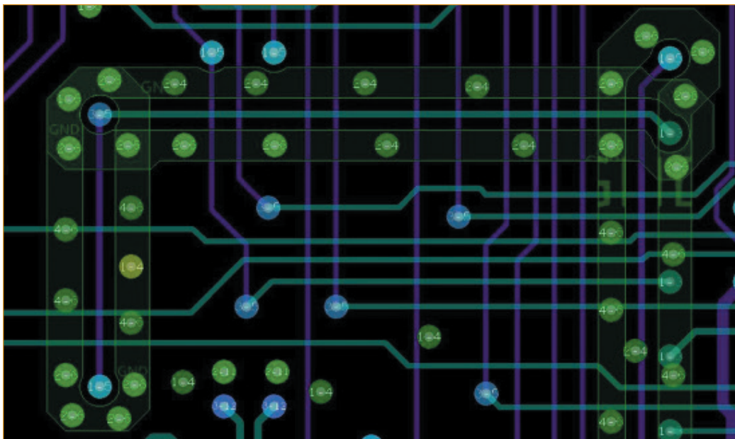
FIGURE 4. The vertical trace on the left (magenta) and the horizontal continuation (cyan) show how to create a guard-band around particularly noisy connections used by externally clocked devices.
