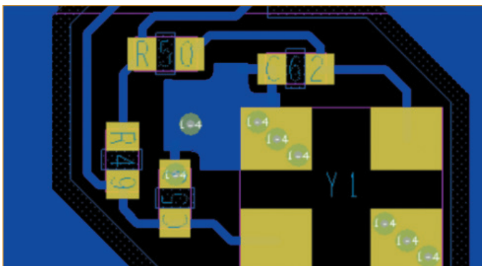
FIGURE 2. It would have been cleaner to rotate Y1 and align the passive elements. We compromised to fit inside the EMI shield.
