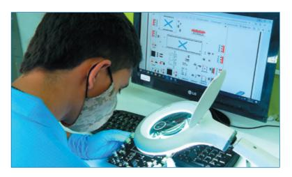
FIGURE 4. Inspecting a PCBA at ColCircuitos.
