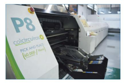
FIGURE 3. The largest EMS in Colombia, ColCircuitos has six SMT lines.
