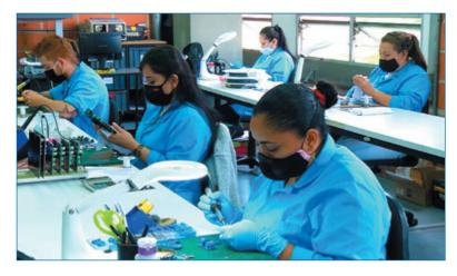
FIGURE 5. ColCircuitos workers perform post-assembly touchup.
