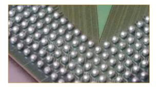
FIGURE 2. Increasing pin density drives the PCB to higher levels of technology. Sequential lamination boards are a mainstream answer in 2021.
