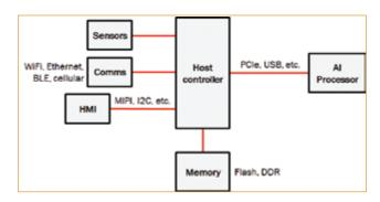
FIGURE 1. High level system block diagram for integrating AI processing into embedded systems.
