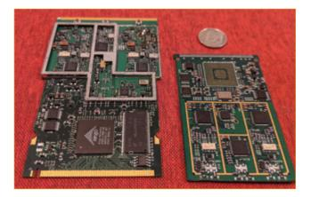
**FIGURE 2.** Generational shrinkage of a WiFi radio over the product lifecycle. They are much smaller these days.
