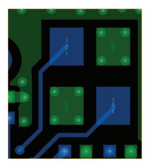
**FIGURE 3.** Isolating a crystal's ground pins from the surrounding copper pour. (I rotated the circuit along with the route-keep-out after this screen grab.)
