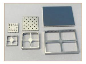
**FIGURE 4.** Off-the-shelf shielding solutions with precut "mouse holes." The crossmembers stiffen the shield walls and provide a central pickup location for automated assembly. The lids can be perforated for airflow. (Source: Laird)
