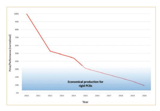
FIGURE 1. Changes in price-to-performance ratio for laser depaneling systems, 2010 to 2020. Source: LPKF
