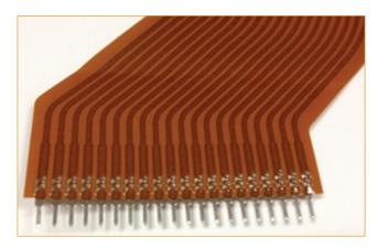
FIGURE 2. IDC contacts pierce through insulation to make contact to copper traces.
