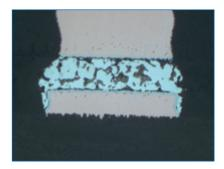
FIGURE 18. Component B, edgebond, 2,129 thermal cycles.
