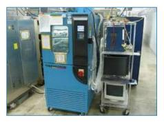
FIGURE 5. Thermal cycling chamber.
