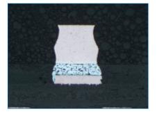
**FIGURE 16.** Component B, edgebond, 1,000 thermal cycles.
