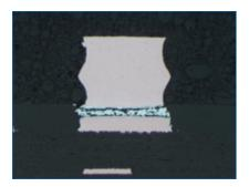
FIGURE 11. Component A, no edgebond, 2,129 thermal cycles.
