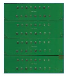
FIGURE 2. Assembled QFN test vehicle.
