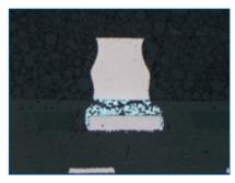
FIGURE 17. Component B, no edgebond, 2,129 thermal cycles.
