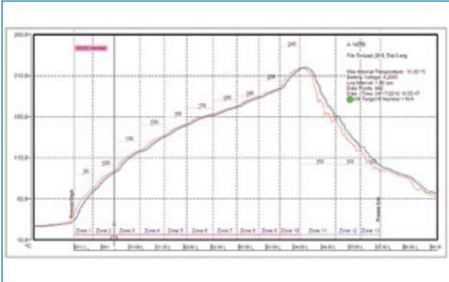
FIGURE 4. Standard tin-lead reflow profile.
