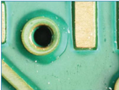
**FIGURE 1.** Solder mask cracking around a through via.
