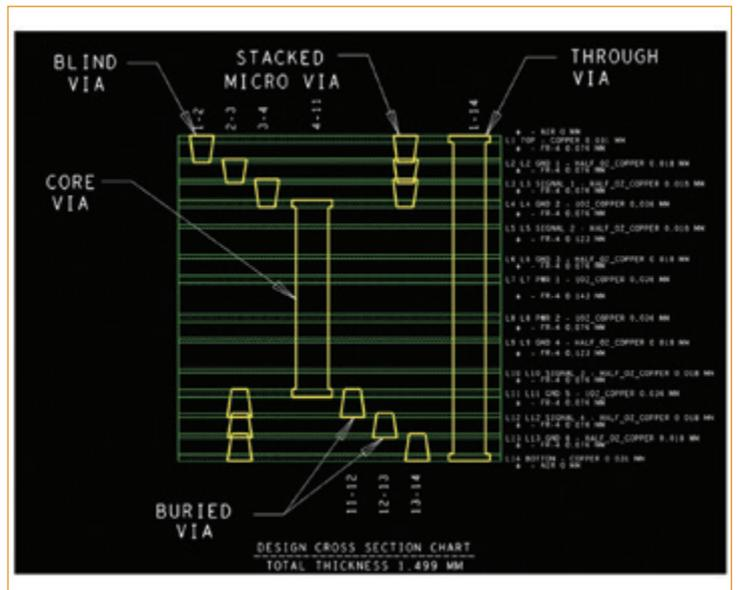
**FIGURE 3.** A 14-layer 3-N-3 stackup, not necessarily to scale.
