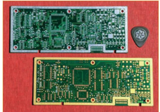
**FIGURE 1.** The DSP side of a mixed-signal PCB. Note that ENIG finish is preferred to HASL of the first iteration above. The via-in-pad flatness improves with gold plating.
