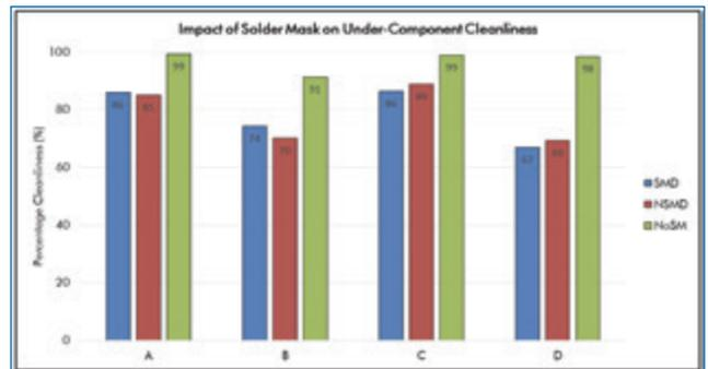
FIGURE 10. Under-component cleanliness: impact of solder mask option.
