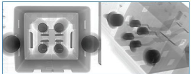
**FIGURE 4.** X-ray images of through-hole components selectively soldered with a low-temperature solder alloy after thermal cycling.
