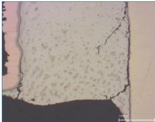
**FIGURE 6.** Microsection vertically through joint shown in Figure 5. Cracking and separation are seen in the bulk of the solder fillet and along the solder joint and plated through-hole interface.
