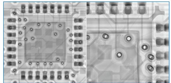
**FIGURE 1.** X-ray images of a QFN soldered onto a PCB using a low temperature solder (LTS).
