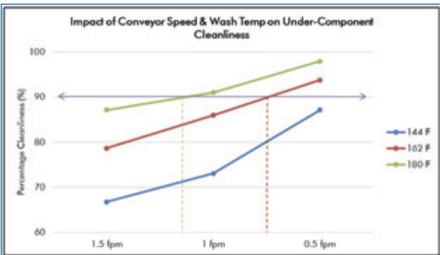
FIGURE 15. Under-component cleanliness: impact of conveyor speed and wash temperature.
