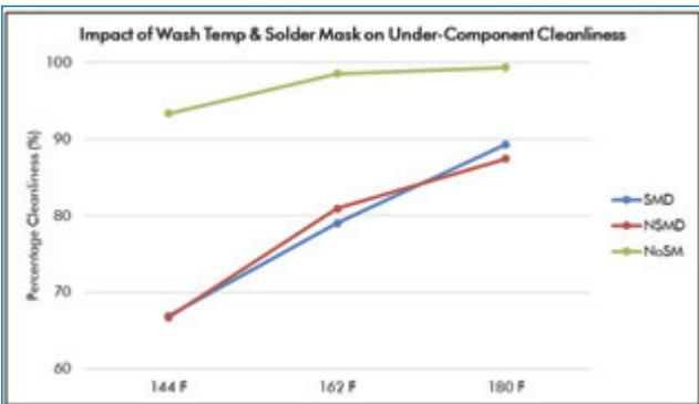
FIGURE 14. Under-component cleanliness: impact of wash temperature and solder mask.
