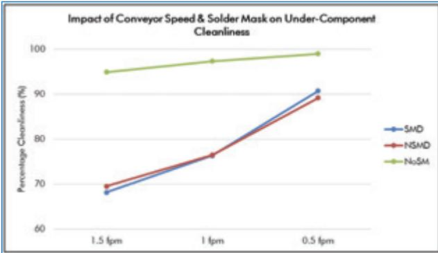
FIGURE 13. Under-component cleanliness: impact of conveyor speed and solder mask.
