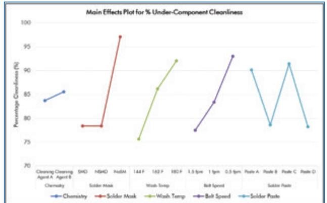
FIGURE 16. Under-component cleanliness vs. process variables.
