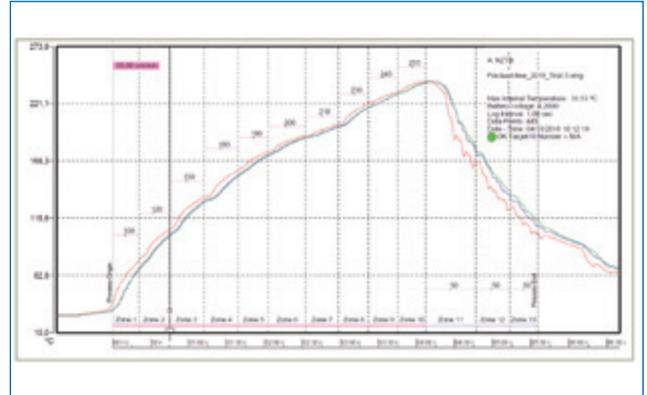
FIGURE 5. Standard lead-free reflow profile.
