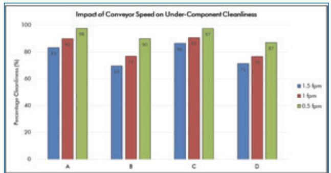
FIGURE 11. Under-component cleanliness: impact of conveyor speed.
