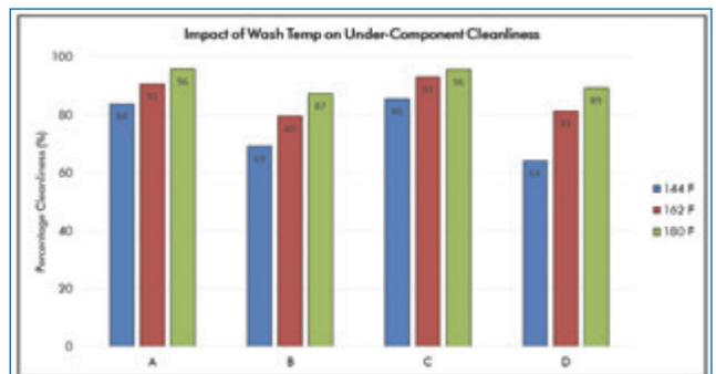
FIGURE 12. Under-component cleanliness: impact of wash temperature.
