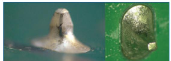
**FIGURE 2.** Optical images of satisfactory through-hole joints produced using selective soldering equipment with a low-temperature solder alloy and following 1,000 thermal cycles.
