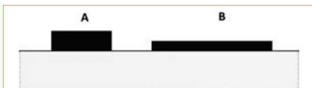
FIGURE 1. Microstrip traces with equal current density can have significantly different temperatures.
