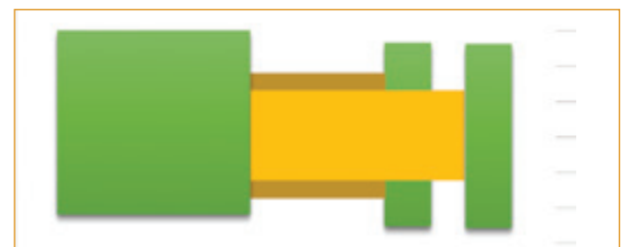
FIGURE 3. If multiple flexes need to exit the main board in the same x-y plane, the main portion of the board needs at least two more layers than the two rigid tails combined.
