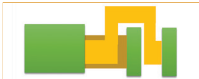
FIGURE 4. By routing one of the flexes around the rigid section of the shorter tail, all three rigid sections can be the same layer count.
