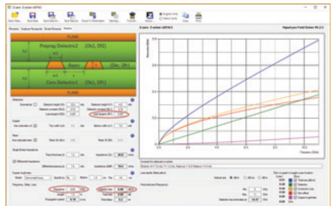
FIGURE 2. Differential insertion loss of 0.60dB/in. computed from a loss tangent of 0.007 at 8GHz using Z-zero Z-planner software and Mentor's HyperLynx field solver.
