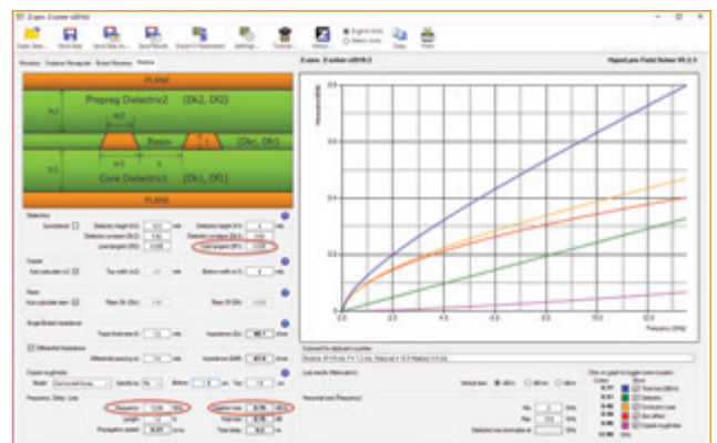
FIGURE 3. A laminate with a published loss tangent (Df) of 0.005 at 12.89GHz results in an insertion loss of 0.75dB/in. per Z-zero Z-planner software and Mentor's HyperLynx field solver.
