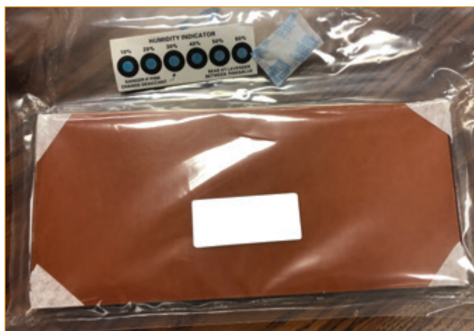
FIGURE 1. Including a desiccant pack and humidity indicator card (HIC) inside the sealed bag will help keep flexible circuits dry when they are on the shelf.
