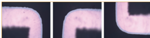
FIGURE 6. Sample 2 RAI gold at 1000X, showing level “0” corrosion/product ratio.
