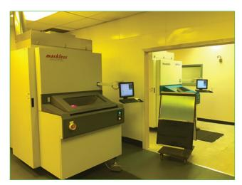
**FIGURE 6.** Recent investments include Maskless Lithography LED direct imagers for solder mark and outerlayer imaging.
