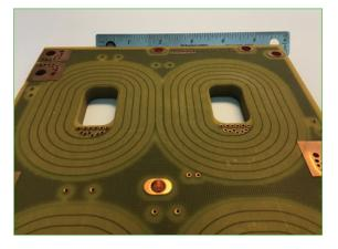
FIGURE 3. ... And this 38-layer solid state rectifier (solder mask removed).
