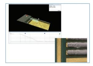
**FIGURE 2.** Nonstandard solder mask steps down to the pad, resulting in poor gasketing and an opportunity for process variation.
