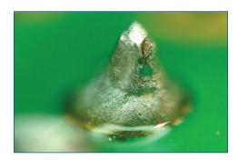
**FIGURE 1.** Connector pin soldered with SnAg using robotic laser.
