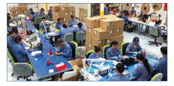
FIGURE 2. The redesigned workcell has a "W" shape that cuts the distance traveled to 5,000 ft.
