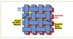
FIGURE 1. Dual-ply glass reduces the probability a trace will be routed over a portion of the glass that has resin-only windows (in yellow) in the glass structure. The second ply, shown in red, serves to reduce the single-ply resin window size and hence glass-weave skew.
