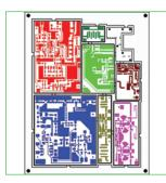
**FIGURE 5.** An actual eightunit layout proposed to a client during quote.
