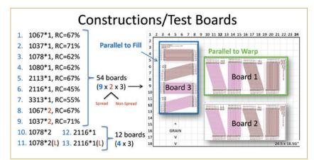
FIGURE 3. Overview of 66 test vehicles in 2015-2016 study of glass-weave skew.
