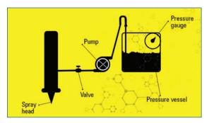
FIGURE 1. Typical pressurized application system.
