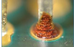
FIGURE 2. Connector pin soldered with SnAg using soldering iron.
