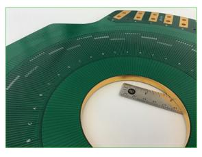
FIGURE 2. Circuit Connect applies its PCB knowledge to non-PCB products, such as this 0.320" heavy copper product with solder mark and gold edge plating ...
