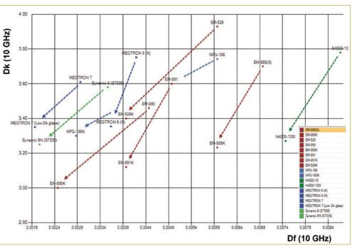
FIGURE 2. A handful of materials from the Z-planner dielectric library that include both an E-glass version of the laminate, as well as a low-Dk glass version. Values are shown at 10GHz and 50% resin content.
