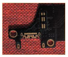
FIGURE 1. It's black over black, but the coverlay openings are visible in this closeup of an FPC with a USB-C connector footprint.
