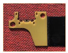
FIGURE 2. FPC from Figure 1, as seen from below. Note the numerous openings for the slots and large holes, while the pin pattern is a mass opening for this stiffener.
