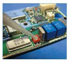
FIGURE 2. A two-component, nickel-filled electrically and thermally conductive epoxy.
