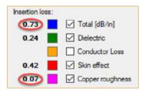
FIGURE 7. Simulation of insertion loss box, showing the comparative contributions of dielectric loss, skin effect, and copper roughness, after switching to  $R_z=1\mu m$  copper. (Source: Z-zero Z-solver software.)
