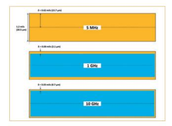
FIGURE 3. Skin depth,  $\delta$  (µm) for a 1-oz. symmetrical stripline trace at three different frequencies.
