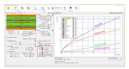
FIGURE 9. The final configuration for our backplane, including dielectric selection based on Dk and Df at 10GHz, dielectric height, trace width, and copper roughness, resulting in 0.55dB/in. (Simulated with Z-zero's Z-solver software.)
