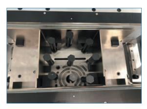
FIGURE 1. High-flow vacuum tooling provides a reconfigurable, lower-cost solution than dedicated tooling plates.
