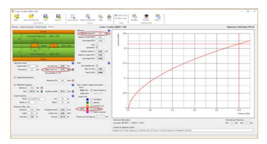
**FIGURE 5.** Resistive insertion loss for a 9.73-mil-wide  $50\Omega$  symmetrical stripline at 10GHz. Simulated with Z-zero Z-solver software using Siemens HyperLynx 2-D field solver.
