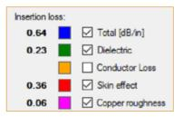
FIGURE 8. Widening the trace by 1 mil reduced resistive loss by 0.06dB/in., and we had to move to a thicker dielectric, 4.5 mils, to maintain our impedance target. (Simulated with Z-zero Z-solver software.)
