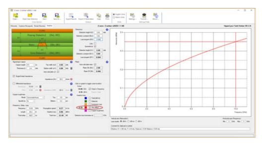
**FIGURE 4.** Resistive insertion loss for a 4.9-mil-wide  $50\Omega$  symmetrical stripline at 10GHz. Simulated with Z-zero Z-solver software using Siemens HyperLynx 2-D field solver.
