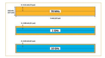
FIGURE 2. Skin depth,  $\delta$  (µm) for a half-ounce symmetrical stripline trace at three different frequencies.
