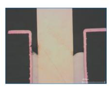
FIGURE 1. Incomplete hole fill.
