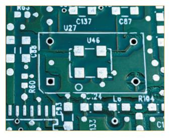
**FIGURE 1.** U27 and U46 are crystals of the same frequency but with different types of packaging. They are mutually exclusive assembly options, depending on the component available.
