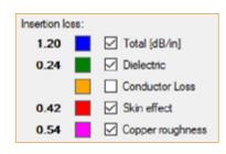
FIGURE 6. Simulation of insertion loss box, showing the comparative contributions of dielectric loss, skin effect, and copper roughness. (Source: Z-zero Z-solver software.)
