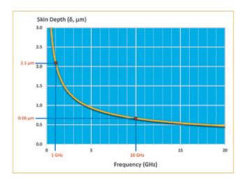
FIGURE 1. Skin depth,  $\delta$  (µm) vs. frequency (GHz).
