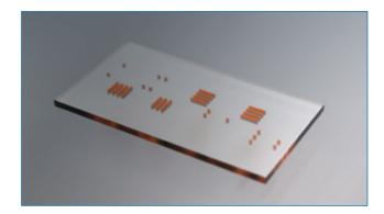
FIGURE 4. Plate and fill cavities with copper.
