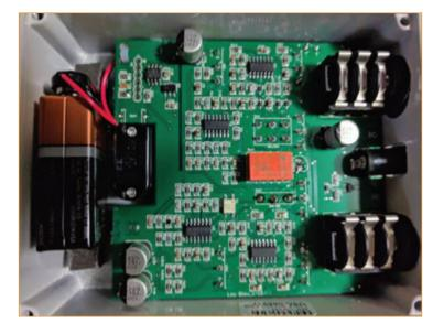
FIGURE 1. Guitar effects pedal small signal processing carried out with the help of basic logic devices.
