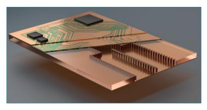
FIGURE 7. Antenna-in-package (AiP) with transmit and receive chips mounted directly to the novel integrated substrate.
