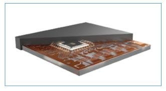
**FIGURE 1.** SIP with integrated passives and wire-bonded IC for fully functional system-in-package.
