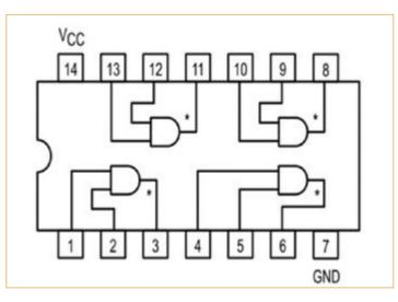
FIGURE 3. 4LS09 QUAD AND GATE typical configuration in a 14-pin package has four logic gates, or six in the case of inverters or buffers. Credit: *Circuit Digest.*
