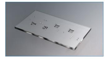
FIGURE 3. Mask, bake and etch PSG for vias, slots or other shapes to form 3-D structures.
