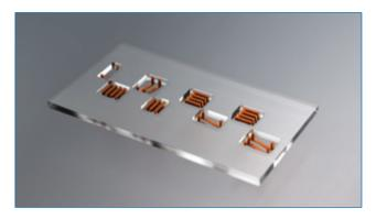
FIGURE 5. Plating of front and backside interconnections.
