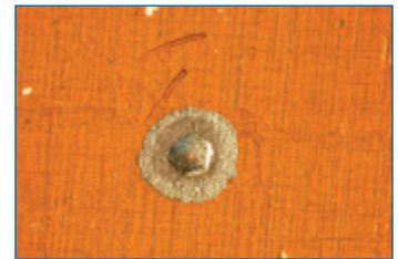
**FIGURE 1.** Solder spots on a NiAu pad (top) and a single spot on a copper OSP pad finish (bottom).
